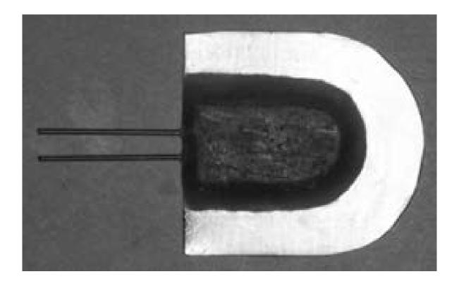
Figure 2: Matrix transfer molding process with one half of mold with velar lamina and wire positioner.
